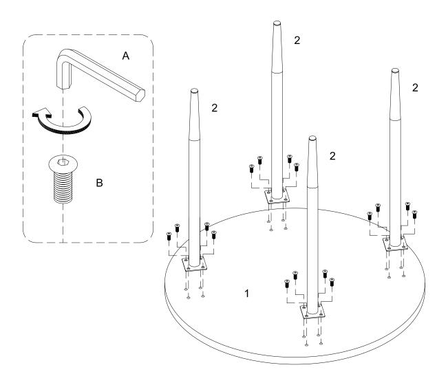
Using bolt (B) attach part (2) into part (1) with hex key (A) as per diagram. Note:Do not tighten all bolts.
