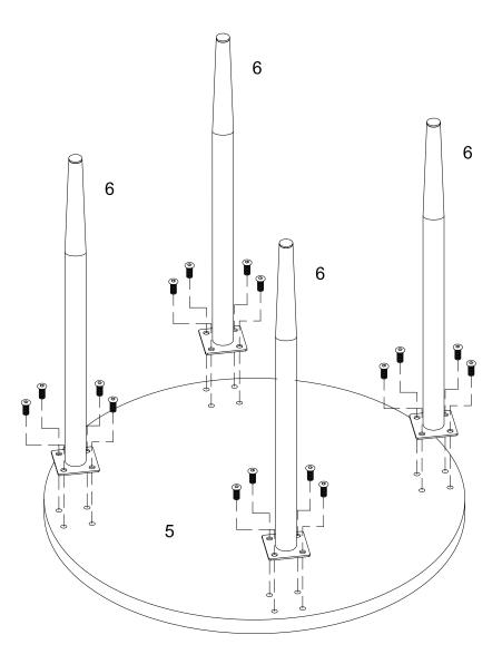
Using bolt (B) attach part (6) into part (5) with hex key (A) as per diagram.
