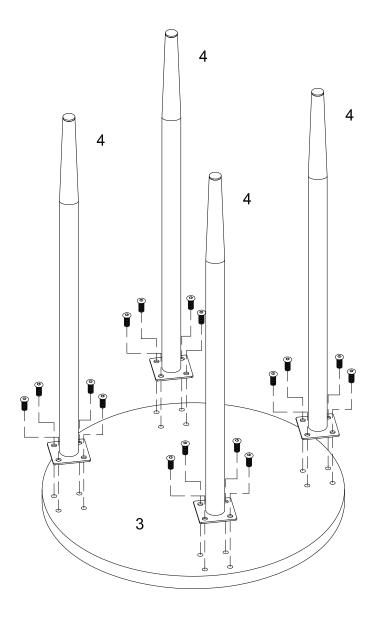
Using bolt (B) attach part (4) into part (3) with hex key (A) as per diagram.
