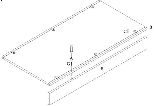
Attach part (8) to part (6) using screw (C) with screwdriver.
