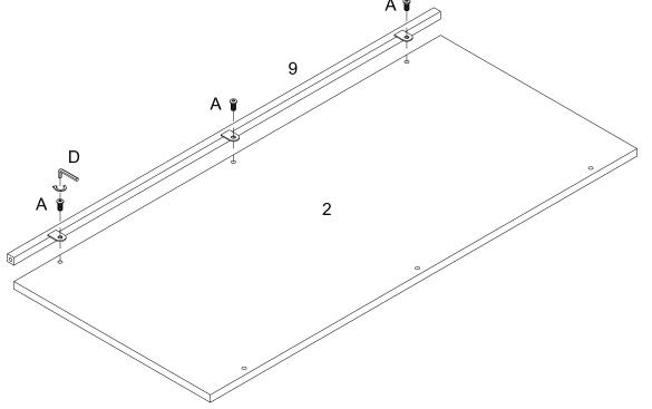
Attach part (9) to part (2) using bolt (A) with hex key (D).
