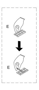
Remove cover tape on glass pads (E), then stick it as diagram.
