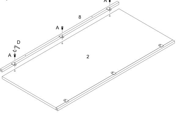
Attach part (8) to part (2) using bolt (A) with hex key (D)
