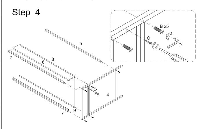
Attach part (4) to part (5,7,8,9) using bolt (B) with hex key (D), and to part (6) using screw
