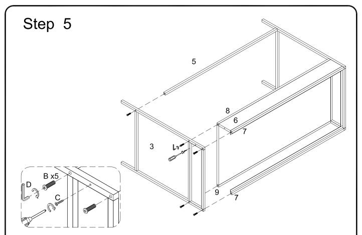
Attach part (3) to part (5,7,8,9) using bolt (B) with hex key (D), and to part (6) using screw (C) with screwdriver.
