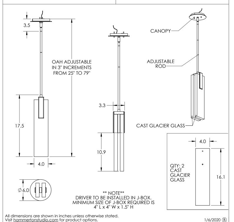
Mounting Packet: Y Weight(lbs.): 19 Electrical Type: CCT: 2700 K LED UL Location: DRY Elec. Qty: 2 Wattage: 5.2 Voltage: 120
