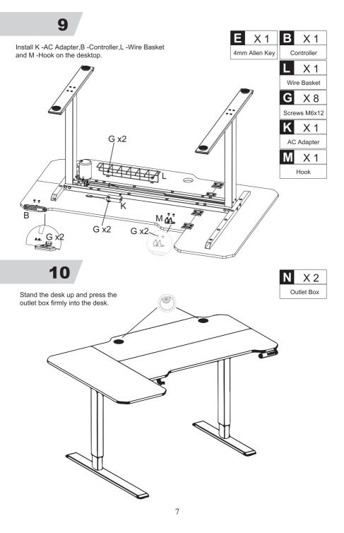
Connect Controller, AC Adapter, Power Cable and Left Leg.
