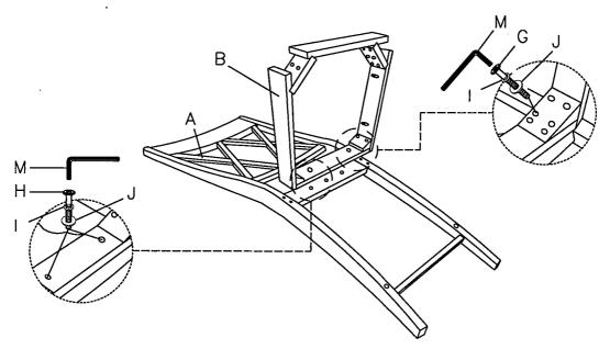
Take the Allen Wrench, and turn the bolts until the legs are secure. DO NOT TIGHTEN COMPLETELY.
