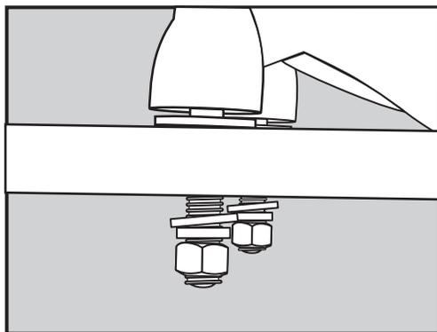
2. Properly align the toilet seat and install the metal washer, metal lock washer and metal nut onto the hinge post.
