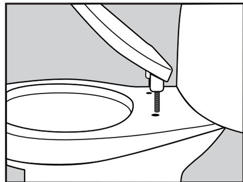
1. Insert the hinge posts into the bowl bolt holes making sure that the soft rubber washer is beneath the hinge and on top of the toilet bowl.
