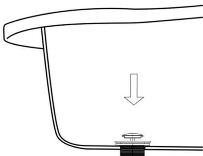
4. Take the lower gasket that was previously removed and re-attach it to the strainer from underneath the bathtub.
