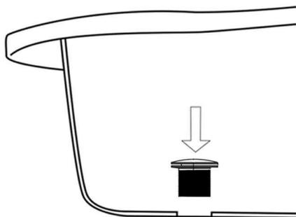
4. Take the lower gasket that was previously removed and re-attach it to the strainer from underneath the bathtub.
