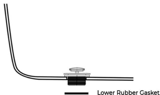
5. Take the drain tee and attach it to the strainer from underneath the bathtub. Tighten as much as possible.
