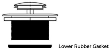
3. Place the strainer through the hole in the interior of the bathtub.
