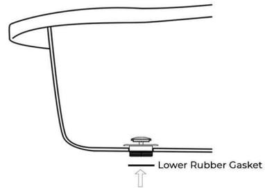
5. Take the drain tee and unscrew the right-handed side cap to connect to the overflow. There will be one gasket that you will remove to use to attach to the overflow drain. Set it aside for now.
