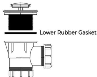
3. Place the strainer through the hole in the interior of the bathtub.
