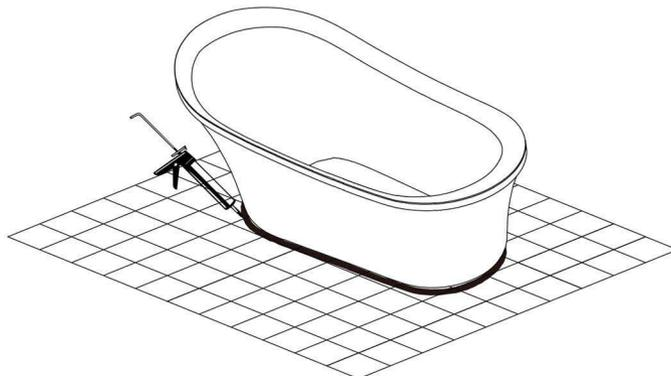
13. With the bathtub now in place, wipe off any excess silicone, tub & tile caulk where the bathtub meets the floor.
