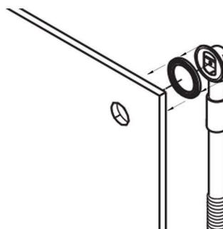
3. Take the overflow plate and place it over the overflow hole. Take the pin bolt and screw it inside to secure it. Take the round overflow cover and screw it onto the pin bolt.
