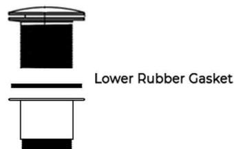
3. Place the strainer through the hole in the interior of the bathtub.
