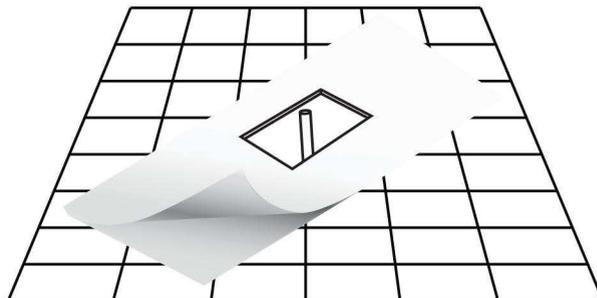
3. Determine the location of the drainpipe on the floor by taking measurements of the drain and waste location underneath the unit. Clean the drain hole area in preparation of setting the drain. The area should be dry & free from any debris.
