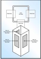
3-Way intersection of fence. A 4-Way intersection would require 2 Posts.
