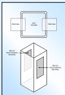
LINE POSTS: Used where two sections of fence meet and are running in a straight line. Some angle variation possible.
