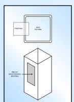
END / GATE POSTS: Used where a fence line starts and ends including when a gate will be installed on any remaining side.
