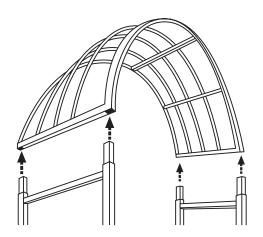
Insert four corners of arch assembly into the four side panel pegs
