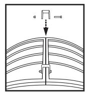
Lock arches together with bracket, bolt and nut (2 places)
