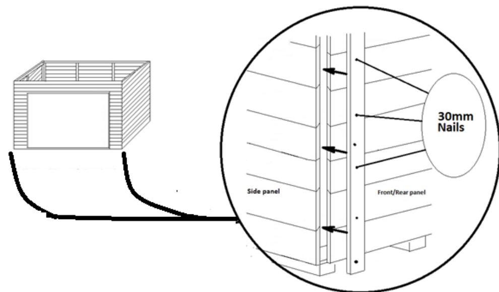
Position the corner cover strips as shown above and fix with 30mm nails.
