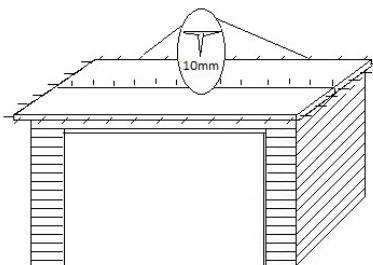
Lay the roof felt with an overhang all round. Fold down the felt at the front and secure using the 10mm clout nails. Tension the felt over the roof and secure to the rear of the roof. Space the clout nail approx. 15cm. Follow the above steps for the sides of the roof. Once the felt is secure trim off any excess.
