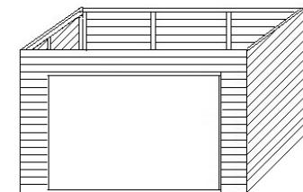
Once all of the side panels are in place, make sure that they are sitting squarely on the floor and fix each side panel to the floor as shown. Use 60mm screws and ensure that the screws go through the floor into the bearers.
