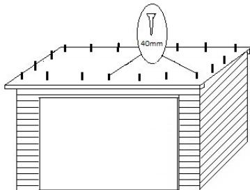
Lay the roof on the shed as shown. Using the 40mm screws, fix the roof into position by screwing through the roof panel into the internal framework of the shed.
