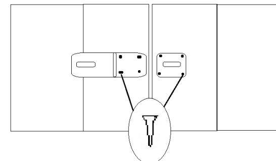
Position the two parts of the hasp & staple across the join in the doors. Make sure that they are both level and will fit together when fixed into place.
