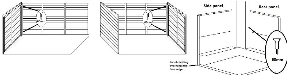
Secure the rear and side panels together as shown below, using 60mm screws. Note that the framework of the panels rests on the floor with the cladding over hanging. Continue until all sides including the front panel are in place and fixed together.
