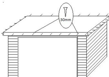
Attach a short barge board to each side of the roof with the 30mm nails, ensuring that the board is flush with the top and front line of the roof.
