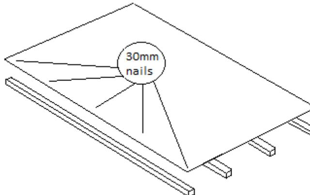
The floor bearers will be either the same length as the width or the depth of the floor.
