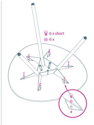
**Step 2** mounting frame to table top: Place the table top so that the "inserts" are visible. Position the frame and fit with bolts and rings. Do not over tighten, this can damage the inserts.
