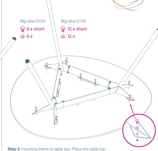
so that the "inserts" are visible. Position the frame and fit with bolts and rings. Do not over tighten, this can damage the inserts.
