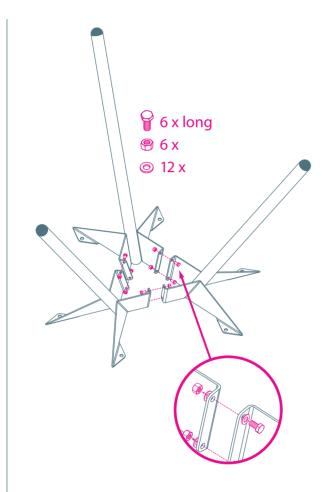
Bolts, nuts and rings needed for assembly.
