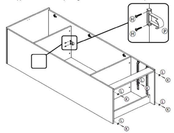
Step 7: Connect the back panels (13) with the spine (14) and secure using hardware part K and a small mallet (not provided).
