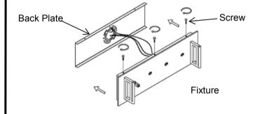
Attach fixture to the back plate, using screws provided.
