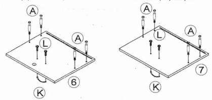
Assemble the Mini Fix(A) to the Drawer Front Panel(6)(7), then install the Handle(K) to the Drawer Front Panel(6),(7)by using Handle Bolt(L) as shown.
