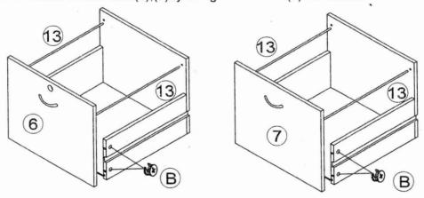
Insert the Iron Rail(13)to the Drawer Back Panel(10), then install the Drawer Front Panel(6),(7) to assemble unit by using Camlock(B).
