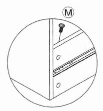
Assemble the drawer to the Runner(F) by using Screw(M) as shown.
