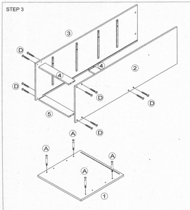
Assemble Bottom Back Cross Bar(5), Cross Bar(4) to Right Side Panel(2) and Left Side Panel(3) by using Screw(D) as shown, then install the Mini Fix(A) to the top Panel (1) as shown.
