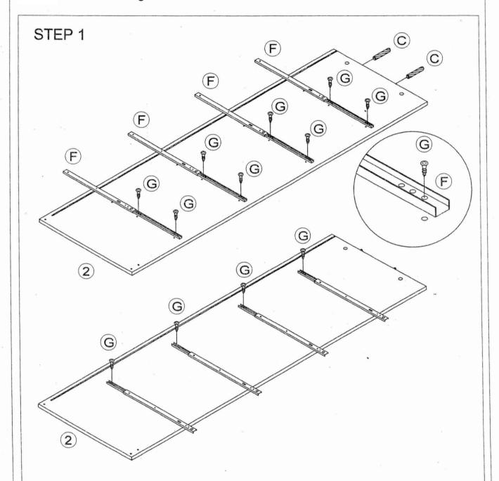
Assemble Runner (F) to the right Panel (2) by using Wooden Dowel(C), Screw(G) as shown.
