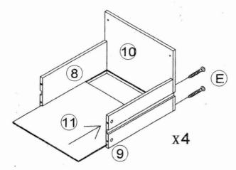
Assemble Drawer Left Side Panel(8), Drawer Right Side Panel(9) to the Drawer Back Panel(10) by using Screw(E) as shown, then insert the Bottom Panel(11) it's position as shown.
