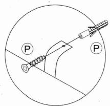
Mount the Wall plug P onto the desired wall location, use screw P to secure the desired spot to prevent the cabinet from falling over as shown.
