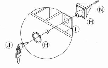
Assemble the Wooden Particle(I) and Lock(H)to the Panel(6) by using Screw(N) as shown.
