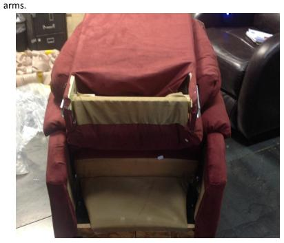
Align the female and male brackets on each side of the back.
